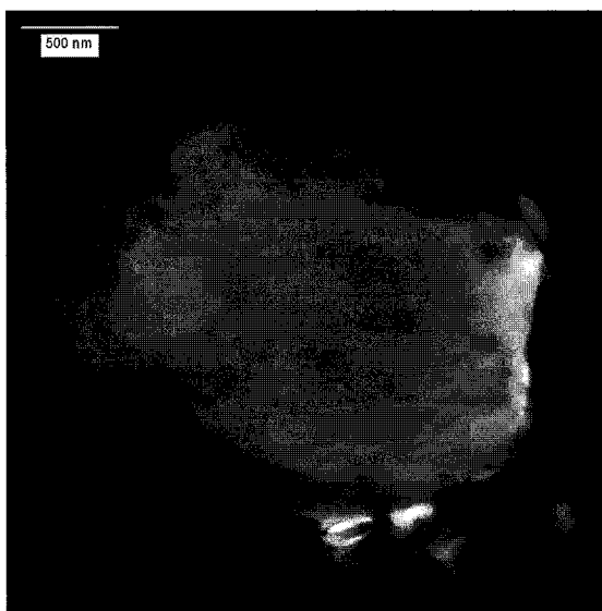
Figure 3. Zero loss filtered TEM image of a PTFE cluster in the PA matrix. Grey zones represent PTFE, black ones indicate PA and bright white areas are due to holes in the sample.
